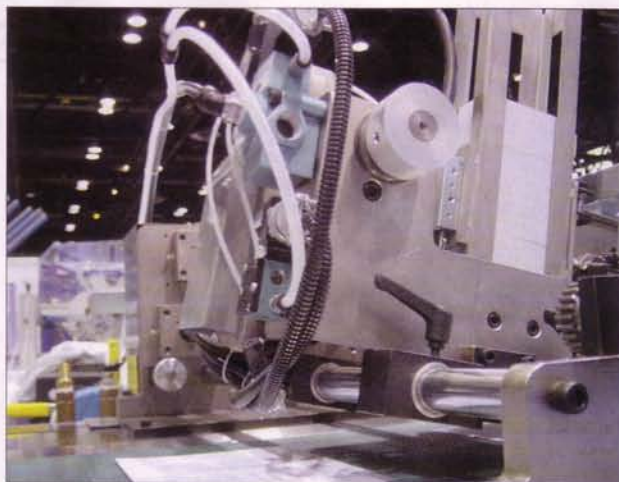
The 912 consists of a vacuum conveying line over which modules can be placed
