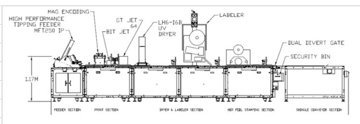
We will be feeding one CR80 card, which has been preperforated into 5 mini cards. Each mini card is then personalised using MEK before verifying data and passing through the hot stamp applicator. Due to its piston design, hot foil labels can run at speeds of up to 250,000 mini cards per hour.
